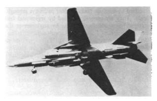
Figure 6-55. Tactical air support. The MiG-23 FLOGGER (above), a variable geometry wing fighter-bomber, is an effective short take-off and landing (STOL) aircraft. The Mig-25 FOXBAT (below) is an all-weather, high-altitude interceptor, easily recognized by its rectangular air intakes on either side of the fuselage.
